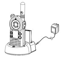
The drop-in charger will also sequentially charge a spare SNN5571 Li Ion battery. The spare battery will not begin to charge until the radio battery is fully charged. Both batteries will charge in approximately 2–6 hours.
